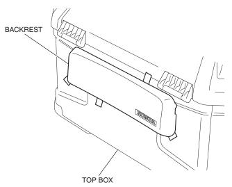
4. Remove the adhesive backing as shown.
