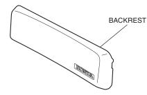
1. Clean the surface of the area shown using an isopropyl alcohol.
