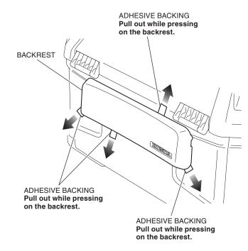
5. Apply adequate pressure to the attached backrest.
